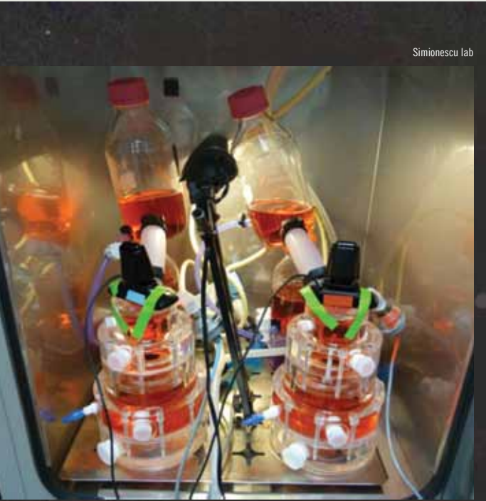
Above: Two heart-valve bioreactors, designed and built at Clemson, work in tandem. Below: A porcine aortic heart valve open and closed in the bioreactor.
